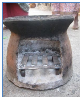
Figure 5 Chulha with the regulator insert
