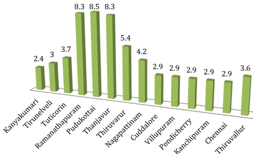
Figure 7 Probable Maximum Storm Surge (PMSS) above tide level in Tamil Nadu districts (Kalsi et al. 2007)
